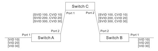
Step 1. Configure Switch A and B.
