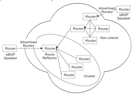
**Figure 8: Connections for Multiple Route Reflectors**
