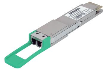
Edgecore’s QSFP-DD 400Gbps transceiver module is designed for optical communication applications over 400 Gigabit Ethernet links of up to 2 km single mode fiber. This product has 8 independent electrical input/output channels that convert 50Gbps (PAM4) electrical input data to 4 channels of 100Gbps (PAM4) optical signals. The electrical interface of the module is compliant with the 400GAUI-8 interface as defined by IEEE 802.3bs, and compliant with QSFP-DD MSA.
