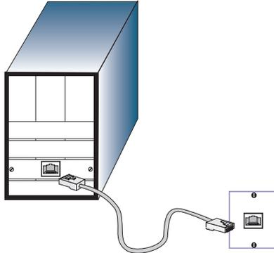
2. If the device is a PC card and the switch is in the wiring closet, attach the other end of the cable segment to a modular wall outlet that is connected to the wiring closet. (See "[Network Wiring Connections](#)" on page 47.) Otherwise, attach the other end to an available port on the switch.
