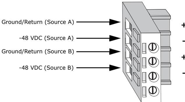
7. Push each wire about half an inch into the opening on the plug, and tighten down the clamp screw securely. You should not be able to pull on the wire and dislodge it.
