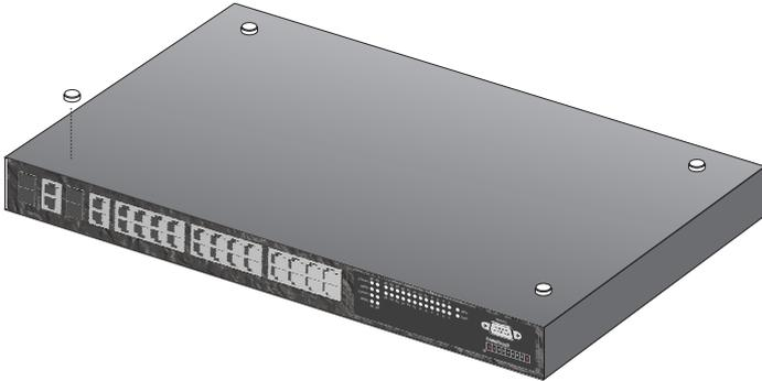
2. Set the device on a flat surface near an AC power source, making sure there are at least two inches of space on all sides for proper air flow.
