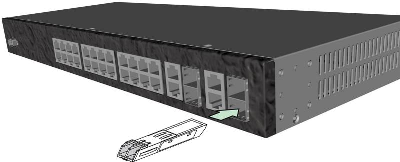
The switch supports 1000BASE-SX, 1000BASE-LX, 1000BASE-LH and other SFP-compatible transceivers. To install an SFP transceiver, do the following:
