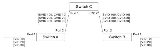
Step 1. Configure Switch A and B.
