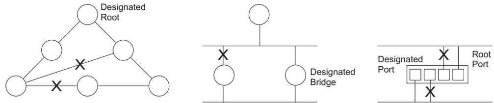
Once a stable network topology has been established, all bridges listen for Hello BPDUs (Bridge Protocol Data Units) transmitted from the Root Bridge. If a bridge does not get a Hello BPDU after a predefined interval (Maximum Age), the bridge assumes that the link to the Root Bridge is down. This bridge will then initiate negotiations with other bridges to reconfigure the network to reestablish a valid network topology.
