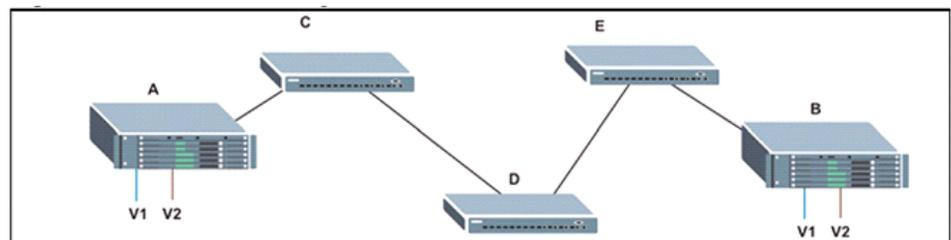
Without VLAN trunking, you would have to configure VLANs 1 and 2 on all intermediate switches – C, D and E; otherwise these switches would drop any frames with unknown VLAN group tags. However, by enabling VLAN trunking on the intermediate switch ports along the path connecting VLANs 1 and 2, you only need to create these VLAN groups in switches A and B. Switches C, D
