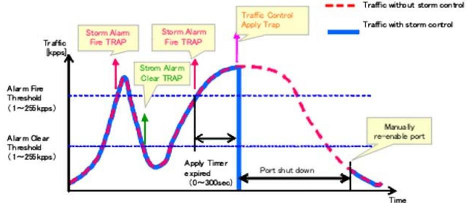
The key elements of this diagram are the same as that described in the preceding diagram, except that automatic release of the control response is not provided. When traffic control is applied, you must manually re-enable the port.
