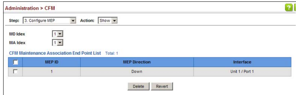
Figure 326: Showing Maintenance End Points
