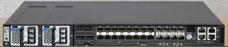
The Edgecore CSR320 is an open design cell site gateway platform that provides a combination of 1/10 Gbps, 25 Gbps, and 100 Gbps interfaces, utilizing merchant silicon and an x86 processor with optimized performance for service provider access and aggregation networks.
