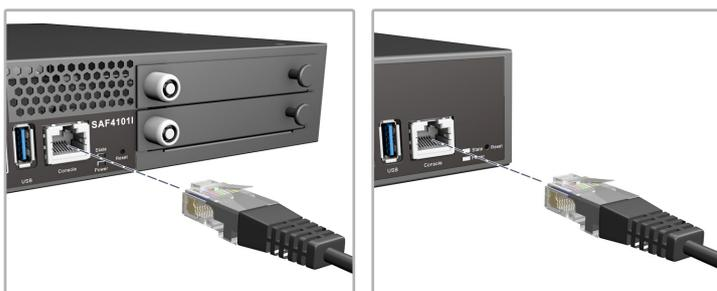
1. Connect a PC to the serial console port using the included console cable.
