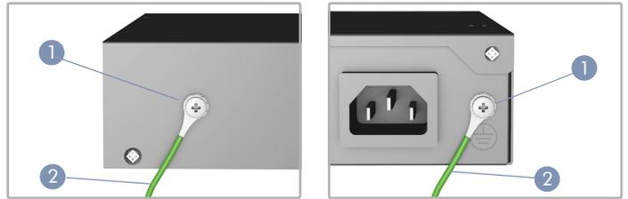
1. Ensure the rack is properly grounded and in compliance with ETSI ETS 300 253. Verify that there is a good electrical connection to the grounding point on the rack (no paint or isolating surface treatment).
