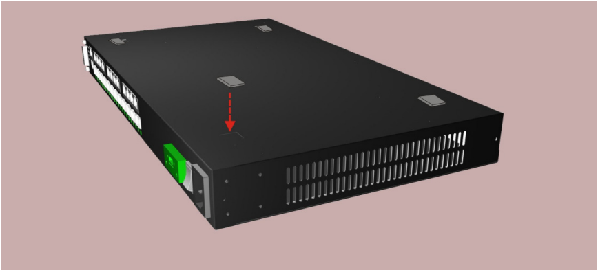
Figure 7: Attaching the Adhesive Feet
