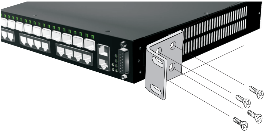
Figure 8: Attaching the Brackets
