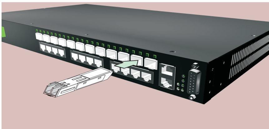
Figure 10: Installing an Optional SFP Transceiver
