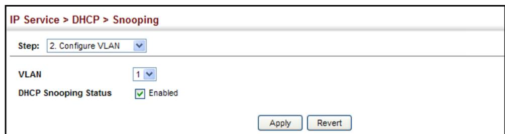
The screenshot shows a web interface for configuring DHCP Snooping. The breadcrumb navigation is "IP Service > DHCP > Snooping". Below the navigation, there is a "Step:" dropdown menu set to "2. Configure VLAN". The main configuration area has two rows: "VLAN" with a dropdown menu set to "1", and "DHCP Snooping Status" with a checked checkbox and the text "Enabled". At the bottom right, there are two buttons: "Apply" and "Revert".
