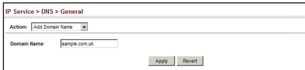
The screenshot shows a web interface for configuring DNS. The breadcrumb navigation is "IP Service > DNS > General". Below the navigation, there is an "Action:" label followed by a dropdown menu with "Add Domain Name" selected. Below that, there is a "Domain Name" label followed by a text input field containing "sample.com.uk". At the bottom right of the form, there are two buttons: "Apply" and "Revert".
