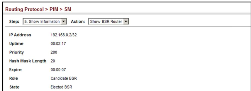
The screenshot shows a web interface for displaying BSR information. The breadcrumb path is "Routing Protocol > PIM > SM". The "Step" dropdown is set to "5. Show Information" and the "Action" dropdown is set to "Show BSR Router". The displayed information is as follows:
