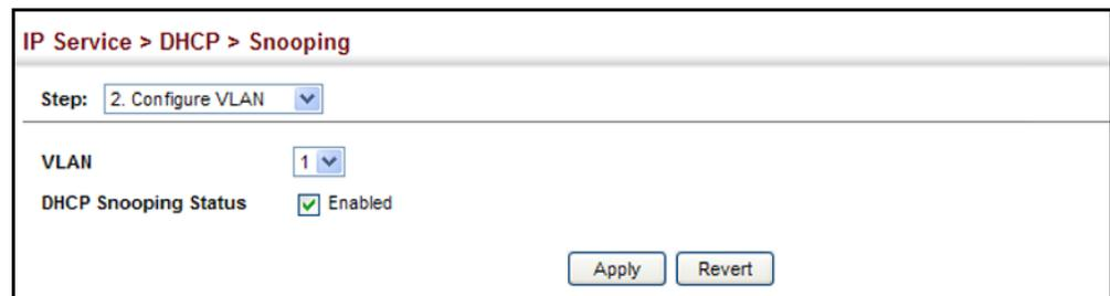
The screenshot shows a web interface for configuring DHCP Snooping. The breadcrumb navigation is "IP Service > DHCP > Snooping". The "Step:" dropdown menu is set to "2. Configure VLAN". Below this, there is a "VLAN" dropdown menu set to "1". The "DHCP Snooping Status" is checked and labeled "Enabled". At the bottom right, there are two buttons: "Apply" and "Revert".
