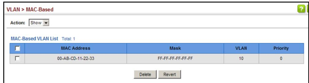
The screenshot shows a web interface for configuring VLANs. At the top, it says "VLAN > MAC-Based". Below that is an "Action:" dropdown menu set to "Show". Underneath is a section titled "MAC-Based VLAN List Total: 1". This section contains a table with the following data:
