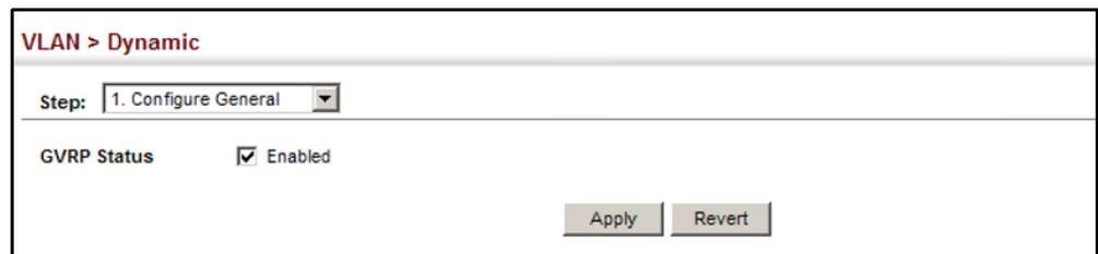
To configure GVRP status and timers on a port or trunk:
