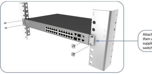
Attach the brackets to the switch, then use the rack mounting screws supplied with the rack to secure the switch in the rack.
