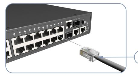
Connect Category 5 or better cables with RJ-45 plugs to the RJ-45 ports.
