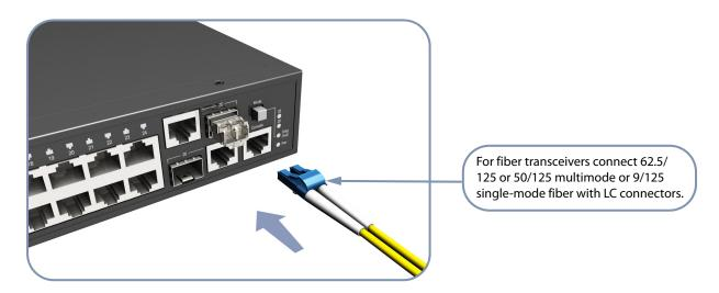
As connections are made, check the port status LEDs to be sure the links are valid.
