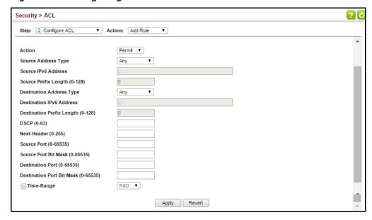
Configuring a Use the Security > ACL (Configure ACL - Add Rule - MAC) page to configure a MAC MAC ACL ACL based on hardware addresses, packet format, and Ethernet type.
