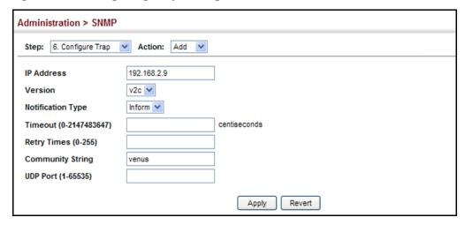
**Figure 244: Configuring Trap Managers** (SNMPv3)
