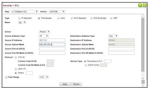
Figure 181: Configuring an Extended IPv4 ACL
