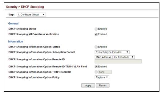
**DHCP Snooping** Use the Security > DHCP Snooping (Configure VLAN) page to enable or disable VLAN Configuration DHCP snooping on specific VLANs.
