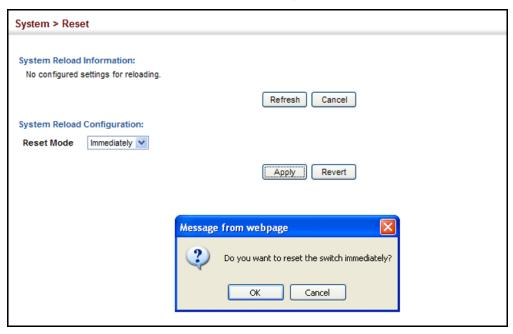
Figure 27: Restarting the Switch (In)
