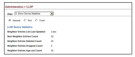
Figure 224: Displaying LLDP Device Statistics (Port)
