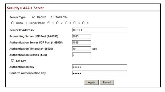
**Figure 146: Configuring Remote Authentication Server** (TACACS+)
