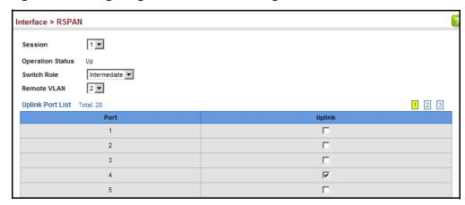
Figure 67: Configuring Remote Port Mirroring (Destination)
