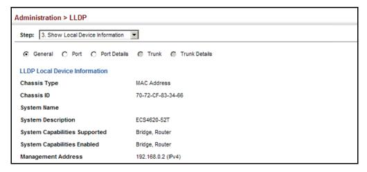
Figure 218: Displaying Local Device Information for LLDP (Port)
