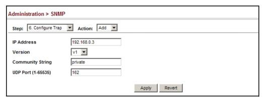
**Figure 243: Configuring Trap Managers** (SNMPv2c)
