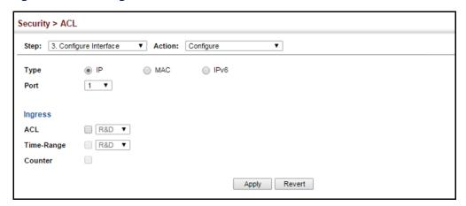
**Showing ACL** Use the Security > ACL > Configure Interface (Show Hardware Counters) page to **Hardware Counters** show statistics for ACL hardware counters.
