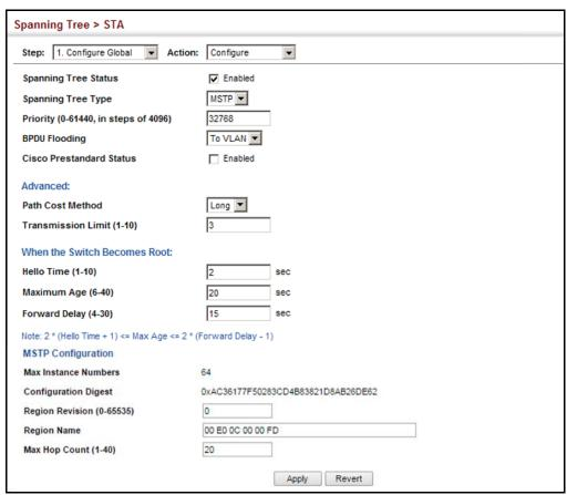
**Figure 107: Configuring Global Settings for STA** (MSTP)
