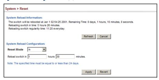
Figure 28: Restarting the Switch (At)
