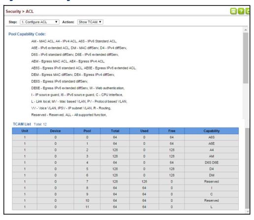
**Figure 177: Showing TCAM Utilization**
