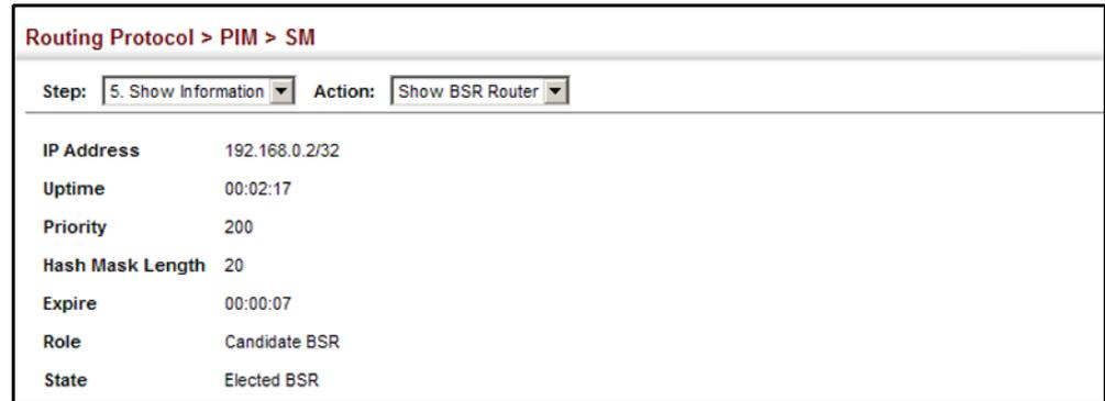
The screenshot shows a web interface for configuring PIM. The breadcrumb is "Routing Protocol > PIM > SM". Below the breadcrumb, there are two dropdown menus: "Step:" with "5. Show Information" selected, and "Action:" with "Show BSR Router" selected. Below these are several parameters listed in a table-like format:
