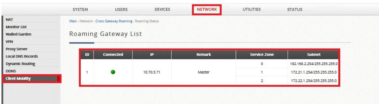
\*\* From this figure, Cross Gateway Roaming has been established between the Master and Slave Controllers. Service Zones enabled on the Master Controller will be displayed.
