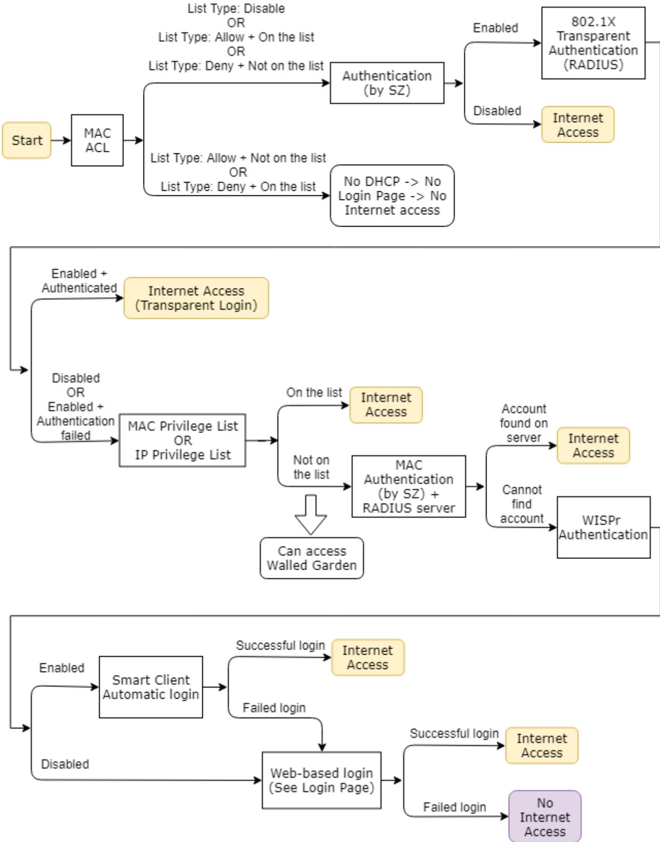
As can be seen from the flowchart, the authentication flow on the controller goes in the general order of **MAC Access Control List > Privilege List > Walled Garden > Non-web Authentication > Web-based Authentication**.
