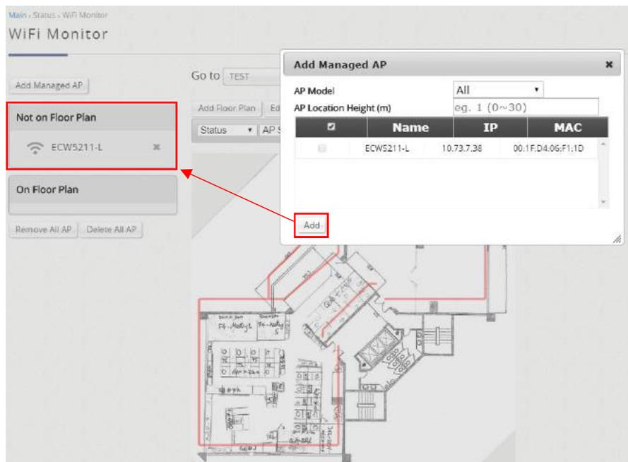
Once these managed APs are created, simply drag and drop these APs onto the floor plan. 2.4GHz is indicated blue and 5GHz is indicated red for signal strength (hence purple when both bands are overlapping).
