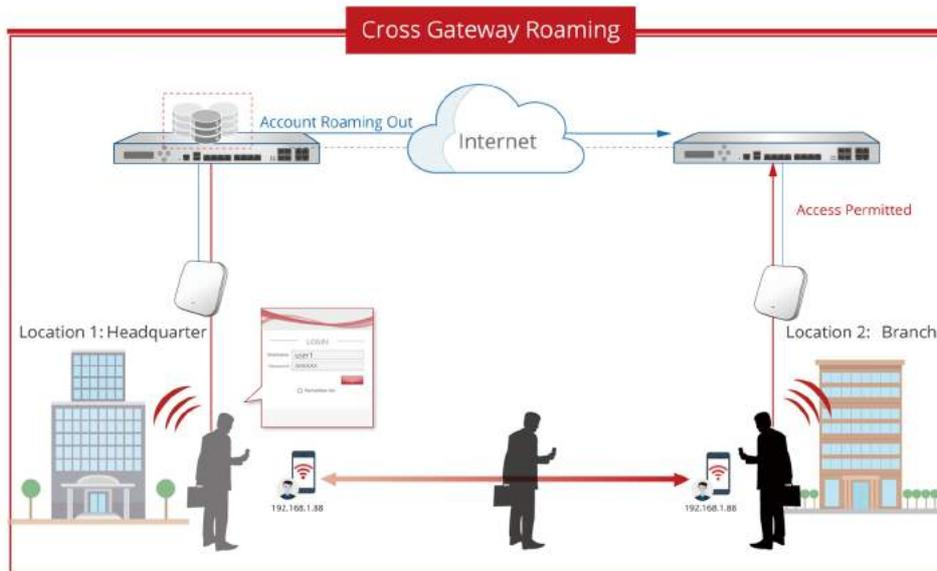
Cross Gateway roaming architecture design adopted is a star topology design where one Master Node may have up to 15 Slave Node peers. The term Master Node simply means that this node takes its place in the center of the star topology.
