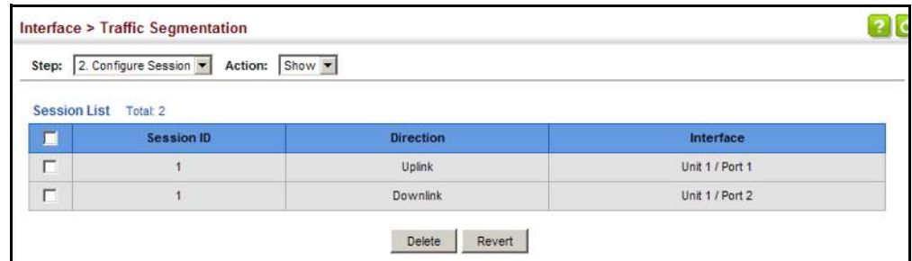
Figure 64: Showing Traffic Segmentation Members
