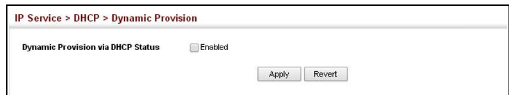
Figure 359: Enabling Dynamic Provisioning via DHCP
