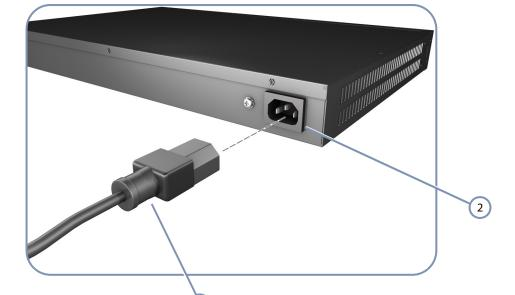
Figure 14: AC Power Cord and Power Socket
