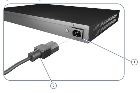
Connect an external AC power source to the AC power socket of the switch using the supplied AC power cord.
