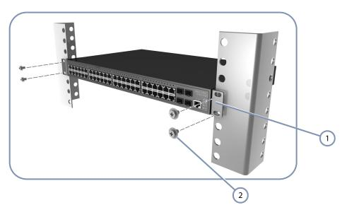
1 Attach the brackets to the switch,
