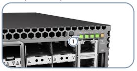
Verify basic switch operation by checking the system LEDs. When operating normally, the PSU1/PSU2, Diag, and Fan LEDs should all be on green.
